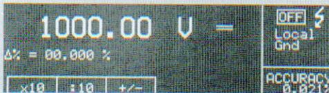
Presence of dangerous voltage over 100 V at the output terminals is always indicated by „Dangerous voltage“ sign. Calibrator indicates dangerous voltage by beeping.
