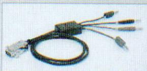
Option 143-60 Cable adapter is designed for simulation of RTD temperature sensors. The adapter is connected to the front panel AUX connector. Platinum and nickel sensors temperature dependency is predefined in the calibrator.
